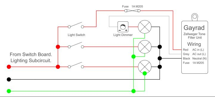
Installation on a circuit with combined light switch and dimmer.
